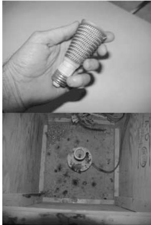
The 600-watt ceramic heat coil [Top] screws into an ordinary porcelain lamp base. [Bottom]
