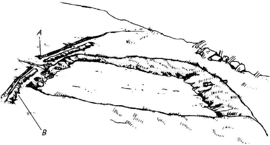
Figure 37: Dike protection by diverting run-off water (Murnyak and Murnyak, 1990). A: ditch; B: dyke.
