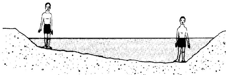
*Figure 25: Cross-section of a pond (Murnyak and Murnyak, 1990).*
