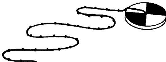
*Figure 11: The Secchi disc (Viveen et al., 1985).*
