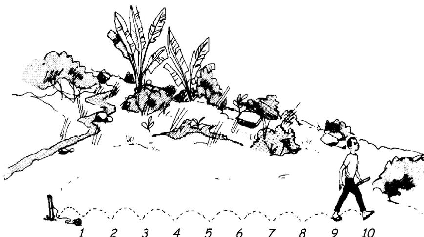
Figure 28: Staking out the pond (Murnyak and Murnyak, 1990).
