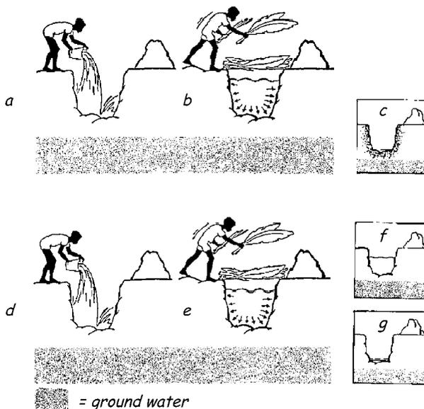
Figure 3: Water permeability test (Viveen et al., 1985).
