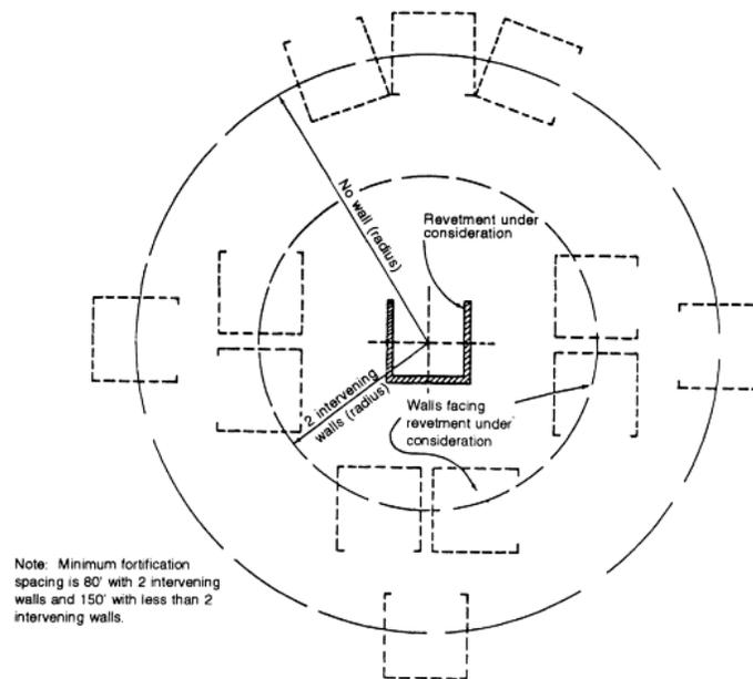
Figure 14-7. Orientation of fortifications to provide safe distances
